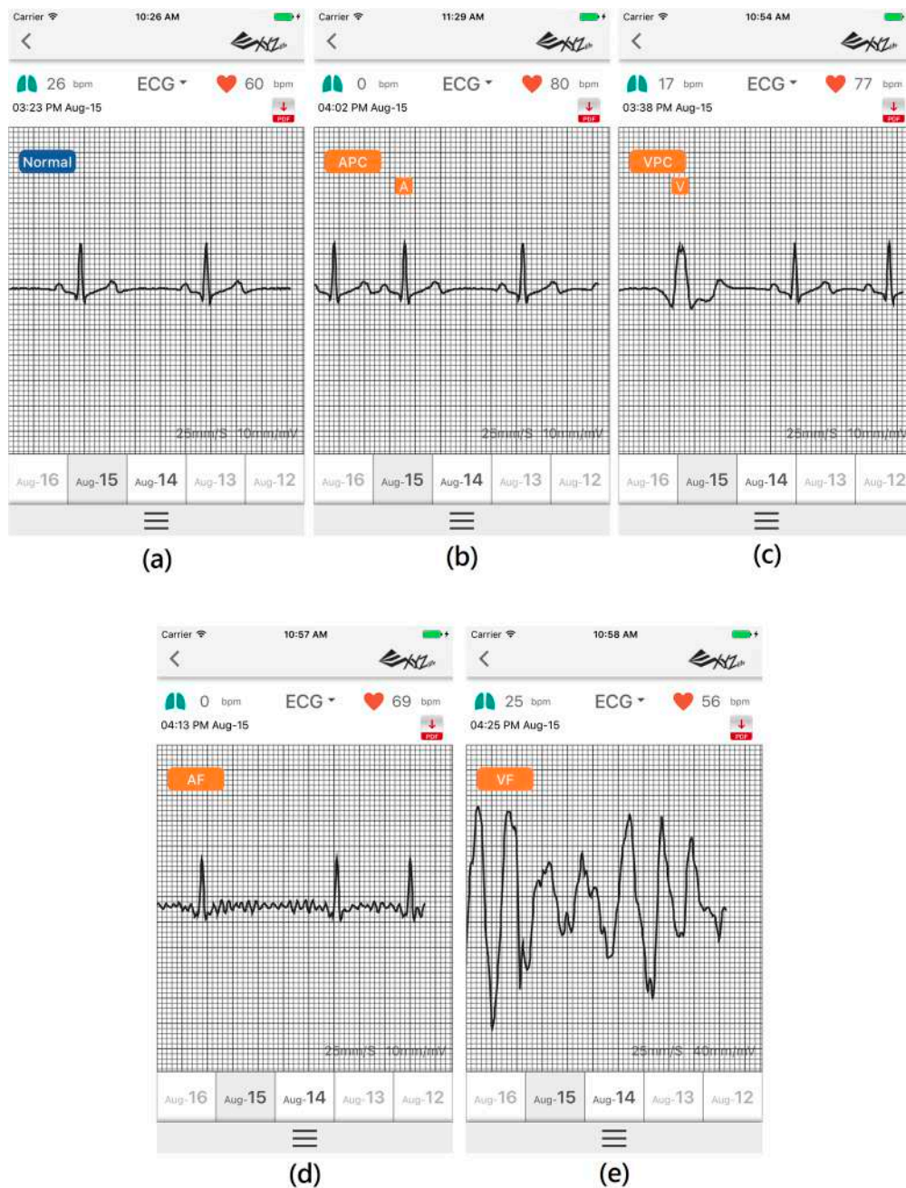
Figure 4. Simulation result from Fluke simulator displayed on mobile phone; (a) Normal sinus rhythm; (b) Atrial Premature Complex (APC); (c) Ventricular Premature Complex (VPC); (d) Atrial fibrillation; and, (e) Ventricular fibrillation.
