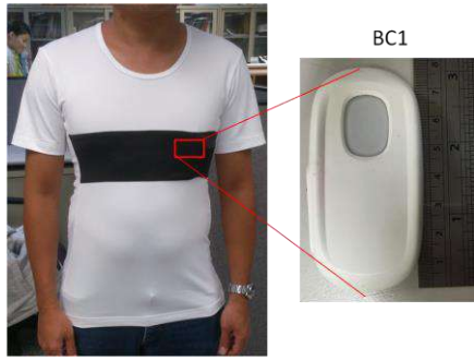
Fig. 1. A fitting clothing with BC1 device, which is placed in front of right chest (red square). Built-in tri-axial accelerometer and gyroscope were used to collect the signal of acceleration and angular velocity.
