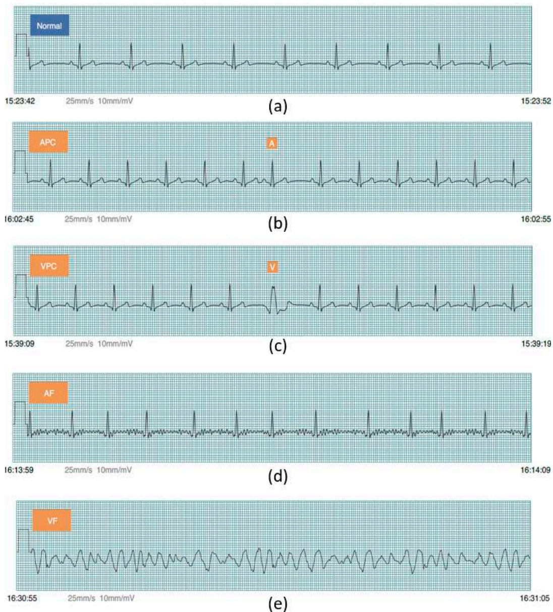
Figure 5. Documented simulation results from Fluke simulator; (a) Normal sinus rhythm; (b) Atrial Premature Complex (APC); (c) Ventricular Premature Complex (VPC); (d) Atrial fibrillation and (e) Ventricular fibrillation.
